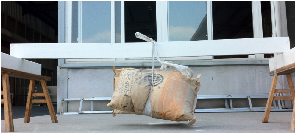
Test Condition: distance=2.6m, loading weight=50kgs, loading time=5min
