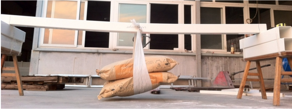
Test Condition: distance=2.6m, loading weight=50kgs, loading time=5min
